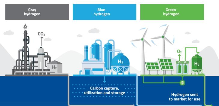
Gray (sometimes called 'brown') hydrogen is produced through fossil fuel processes. The process of producing it releases carbon straight into the atmosphere. Today most hydrogen is produced this way.
