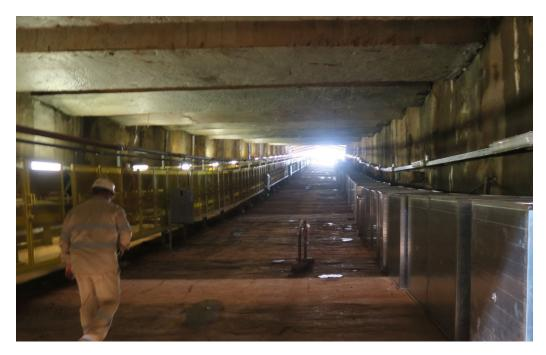
Photo 3. Ramp and Phase 1 conveyor from base of crusher pit leading to secondary sizer
