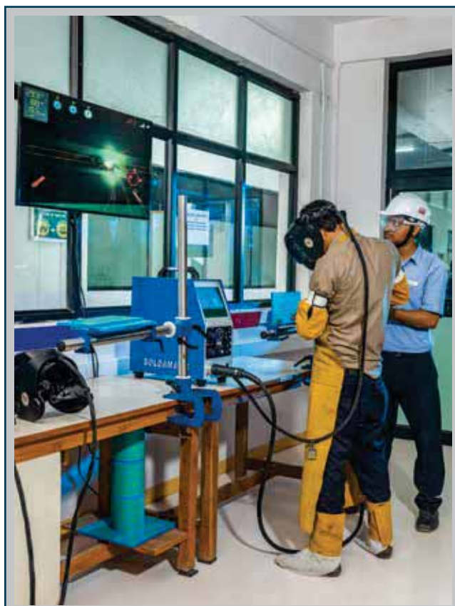
Virtual weld simulator for students to learn welding trade
