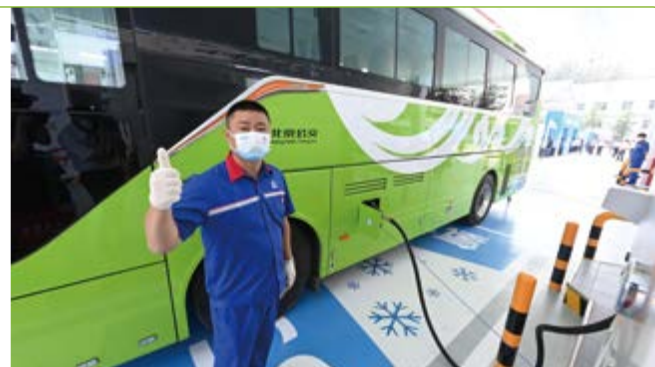
④ In October 2021, Shanghai Petroleum's Qingwei hybrid station was officially completed, which can serve hydrogen vehicles with both 35 MPa and 70 MPa hydrogen fuel cells
