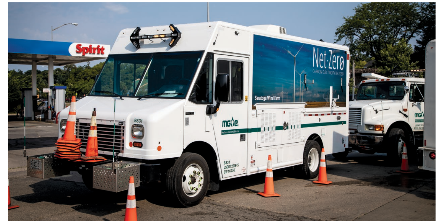
Crews working on MGE's underground electric network system in downtown Madison use this truck with battery-powered auxiliary equipment, which avoids vehicle idling while crews perform their work, helping to reduce emissions and fuel costs.
