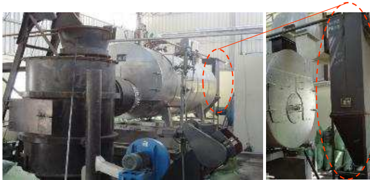
Figure 25: Ceramic Multi-Tubes Precipitator (black color cylinder) to Filter Air Emissions (retain rice husk ash particles from releasing into atmosphere through chimney)
