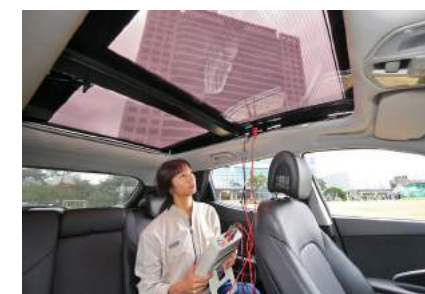
Performance evaluation of the second-generation roof panel
